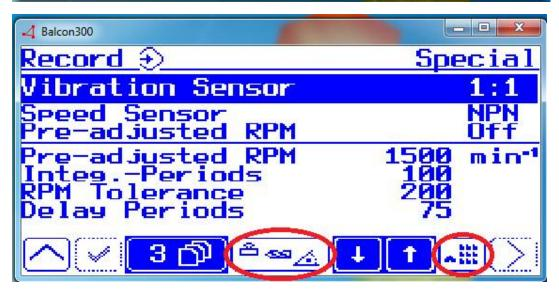
Once the balancing configuration settings have been set (you can change the values using the red circled icon on the right) you may need to change the pitch parameters. These can be accessed by the red circled icon on the left.
