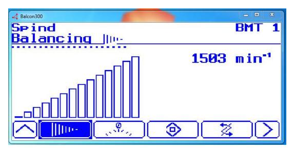
From here you can simply click the balancing icon (in blue) to start running a balancing test. Once finished the following screen will display.
