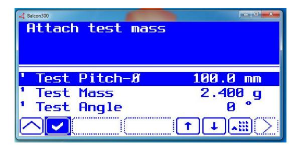
Stop the spindle, add the test mass before restarting the spindle and then click the check icon. Note that you are selecting the zero degree reference by where you are placing the test mass. You'll want to somehow mark this position for reference. It will then take readings and ask you to remove the test mass. Stop the spindle, remove the mass before restarting and click the check icon again. It will then take final readings before showing you the results page.
