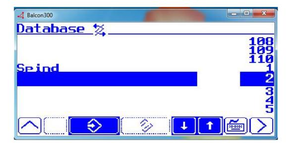
Using the Up/Down arrows from here you can select another wheel/part from the list. As shown above only the spindle has been configured. The name of the wheel can be changed by selecting the keyboard icon.
