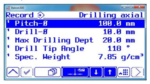
As shown you can adjust the pitch, drill size and also the density of the wheel/hub you are balancing. The default density is for steel (7.85 g/cm3).
