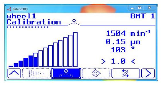
Here you will start the spindle and then click the calibration icon (in blue) to start the test. Once it starts you will be asked to add a test mass:
