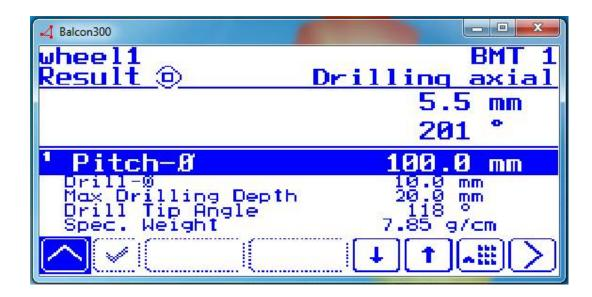
After altering the wheel to be balanced according to the results, you can select the Up arrow on the left to go back to run subsequent balancing tests until you are satisfied with the wheel balance.
