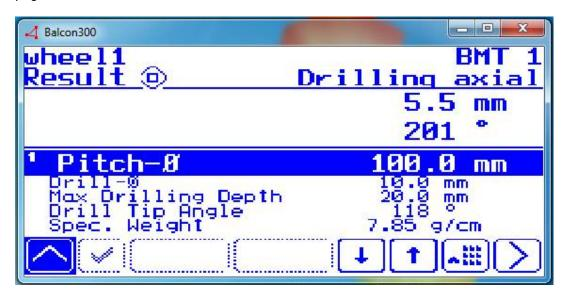
This is the same screen as the balancing result screen shown in the beginning. After modifying your wheel as indicated you can select the Up arrow and run another balance test and continue to do so until you achieve the desired balance result
